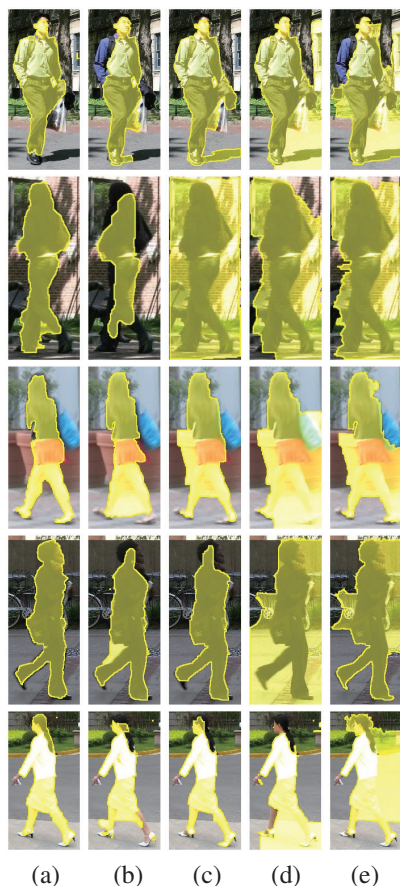
Fig. 9. Comparison between segmentation methods (PennFudan Dataset). (a) Proposed method, (b) SSFseg, (c) One-cut, (d) Grab-cut, (e) Watershed.
